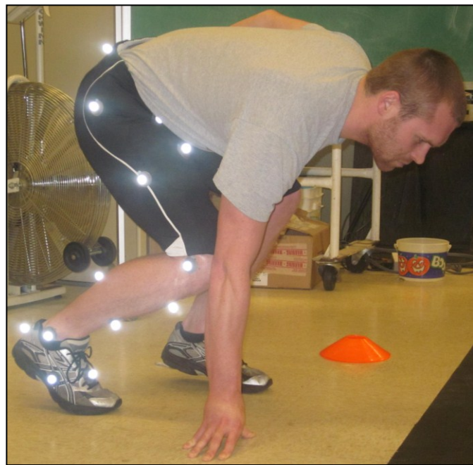
Figure 9: Gait Analysis marker positions on right leg and pelvis
